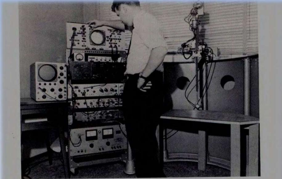
**Figure 11.** An abdominal echoscope constructed in 1962 by G. Kossoff, who is seen in this picture. The transducer is attached to the rack on the right of the photograph, and in clinical use it is immersed in a water tank; the patient is positioned with her back supported by an inclined couch, with her anterior abdominal wall in contact with a flexible membrane that forms one of the walls of the water tank.
