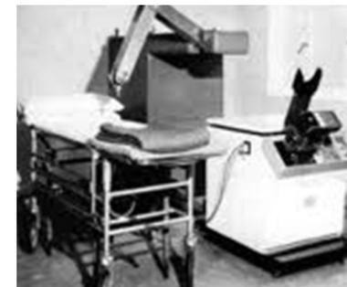
1962 Physionics produced three-jointed articulated-arm handheld scanner in USA
